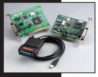
Keithley's GPIB interface solutions make it easy to add standard IEEE-488.2 bus control to any PC. These high speed tools can serve as a talk/listen device or can operate as a system controller, controlling as many as 14 GPIB instruments or other devices over a distance of up to 20 meters. They are ideal for use with automated test equipment in laboratory and industrial applications.
